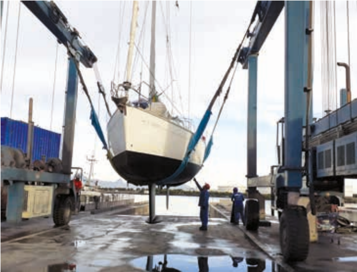
Haul out at Technimarine
