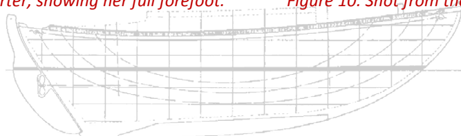
Figure 9: ERIK's underwater shape, from the forward quarter, showing her full forefoot.
