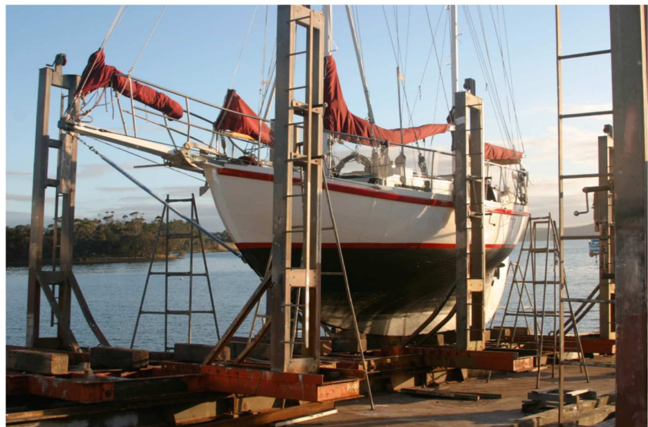
Figure 9: ERIK's underwater shape, from the forward quarter, showing her full forefoot.
