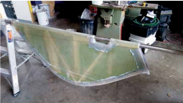
Repairs to the rudder
