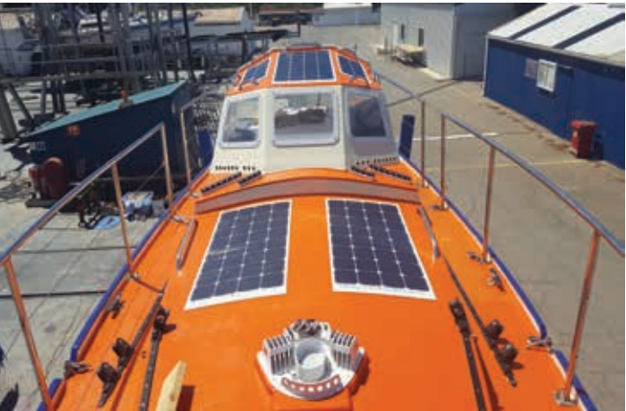
Deck painted to enhance visibility from the air
