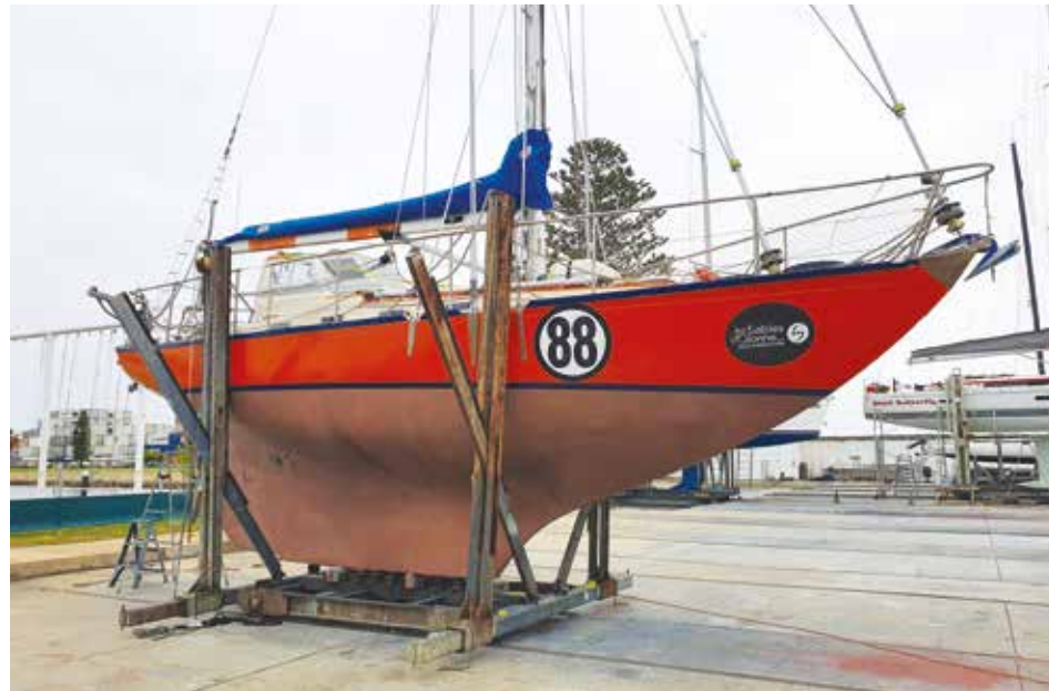
Coconut's topsides refreshed and below the waterline, burnished Coppercoat
