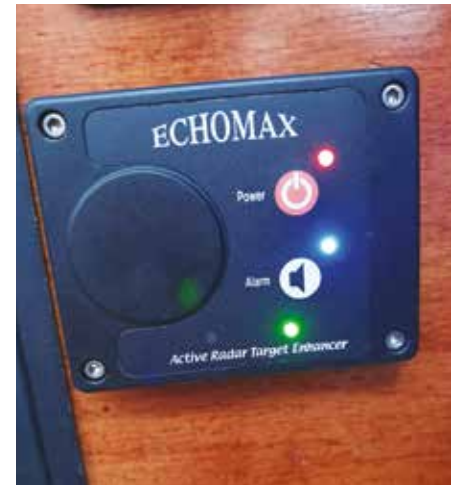
New control box fitted to Echomax active radar target enhancer to provide audible alarm of shipping
