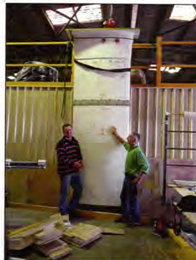
Jeanne Pierre Kerry of Kiki, and Chris Riggs with the new centre board, bulb yet to be fitted. Jeanne has been a stalwart in the rebuild and is currently making beautiful cabinetware for Helsal's interior.
