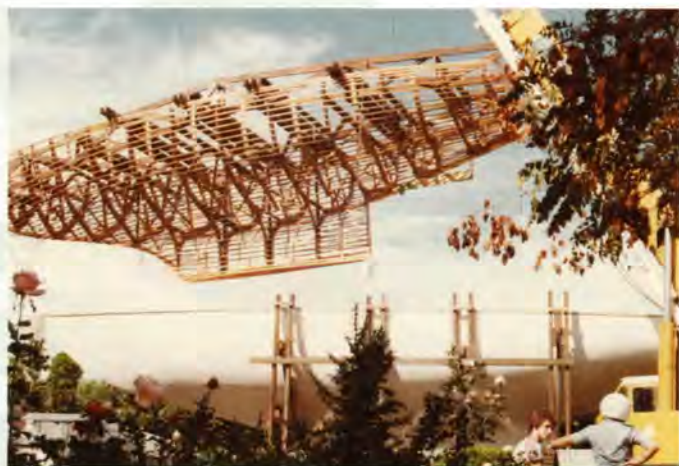
In April 1993, the hull was turned over and the timber plug removed to enable interior glassing.
